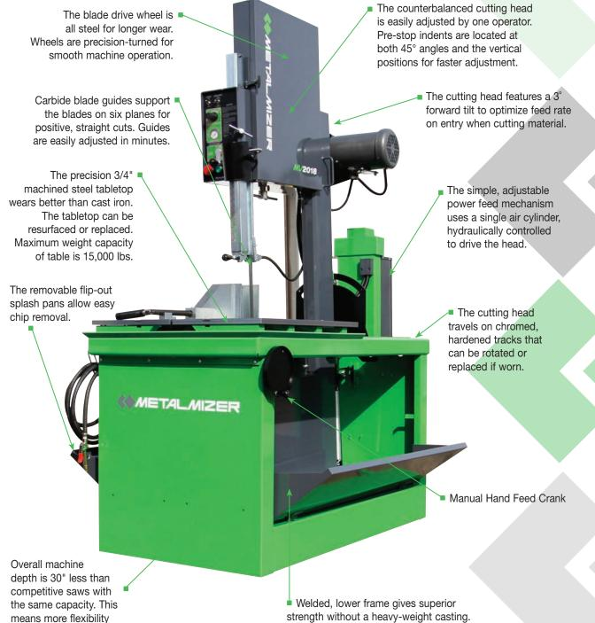
MetalMizer is easier to move and ship.
